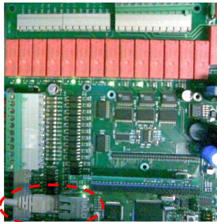
Figure 2 CTS6000 PCB with network port
